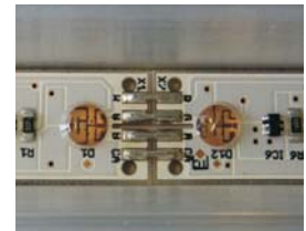
Solder bridges for EasyLED RGB
